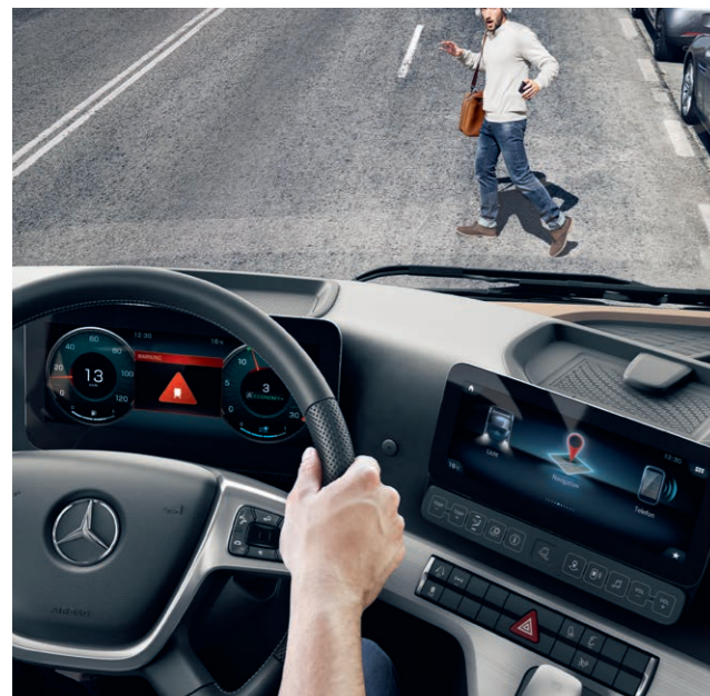
Active Brake Assist 5 1) . By carrying out full brake application, it can reduce the severity of accidents or even prevent them completely.
