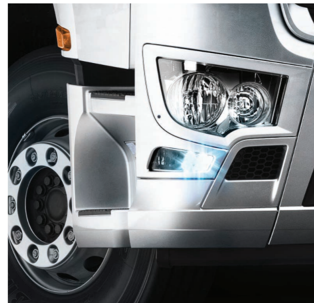
LED day-time running lights. Safety is further enhanced by the standard LED day-time running lights. This also makes the vehicle more visible to other road users.
