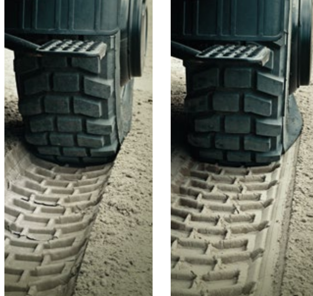
With Tirecontrol you can adjust the tyre pressure to suit the terrain – simply with a switch.
