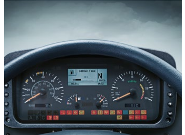
The instrument panel is clearly structured with an easy-to-operate driver information system, backlit dials and two LCD multifunction displays.
