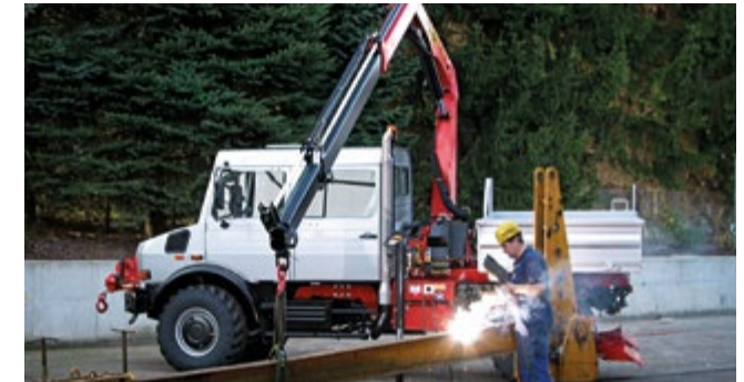
Commercially-available hydraulic pumps, e.g. for a crane, can be used via a standardised connection on the manual transmission.
